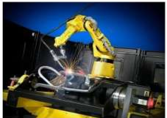
ROBOTIC WELDING MACHINE
